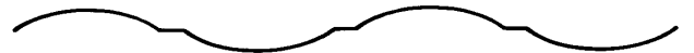
Fig. 21B — Smaller Amplitude Sine Wave with same amount (higher %) of Crossover (notch) Distortion.
